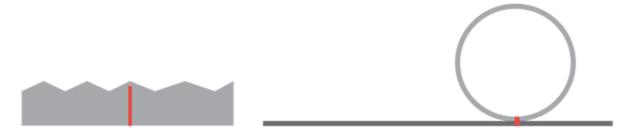
2. Place a mark on the inside of your blade and then place the blade on the ground with the mark lining up with a mark on the ground.
